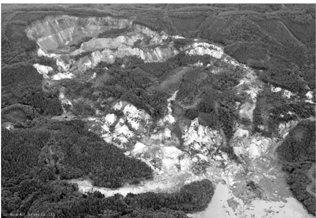
Fig. 2 – A landslide (1.7 km x 0.7 km) triggered by 7.2 magnitude earthquake on 14 June 2008, in Kurihara city, Miyagi Prefecture, taken soon after the event date. The ground surface collapsed consists of young volcanic formations from neighbor volcanoes. Photo courtesy of the Asia Air Survey Co. Ltd.
