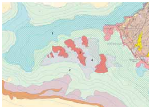
Fig. 1 – Detail of the map at 1:30,000 scale. 1 – Bank; 2 - Slope; 3 – Coralligenous buttresses; 4 – Terrace.
