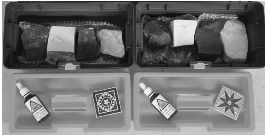
Fig. 1. Example of a multi-kit. Two of a five boxes-set on experimenting the usefulness of the common “test of the acid” (limestone identification through the spontaneous reaction of \text{CaCO}_3 to diluted \text{HCl} ) with two whitish and two blackish rocks, some with positive and others with a negative reaction, independent of its color. Based on rocks typically used on Portuguese sideways.
